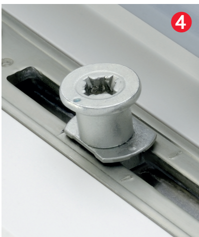
Security locking cams with a mushroom head provide high security in conjunction with security strikers
